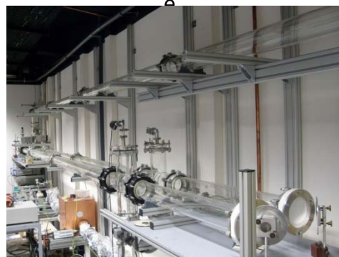
Very long absorption cell for high sensitivity measurements.
